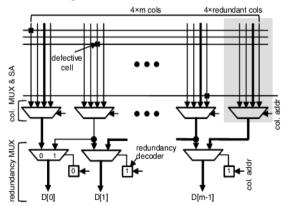
Fig.2 Example of Column Redundancy Implementation in SRAM Array
