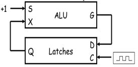
Fig.4 ALU with Latch as memory element
