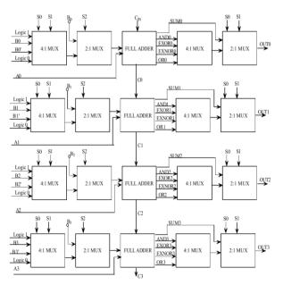
Fig.3 Block Diagram of the 4-bit ALU Design
