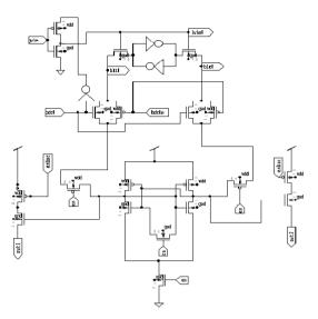
Fig.1 8T CDC with bit line decoupled current sensing amplifier
